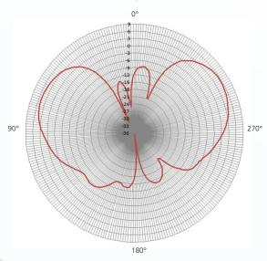
Elevation Polar Radiation Pattern 490 MHz
