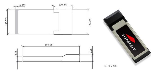
The SDC-EC25N is fully compliant with the PCI Express Card Type 1 mechanical standard. It can therefore be inserted in any Express Card hardware interface and typically does not require any additional mounting hardware.
