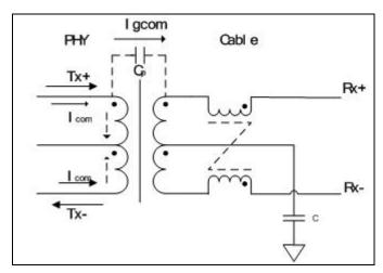
Diagram 7: Ethernet Transformer with a Common Mode Choke
