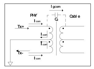
**Diagram 5: Ethernet Transformer Operation Principle**
