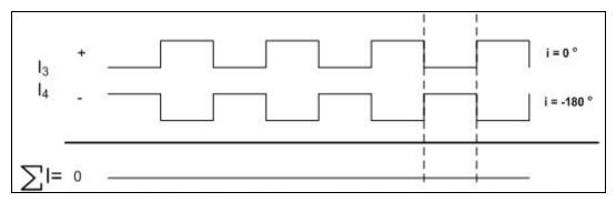
Diagram 3: Phase Different of the Currents and No Current Flow to Ground
