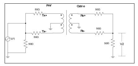
**Diagram 6: Ethernet Transformer CMRR Test Circuit**
