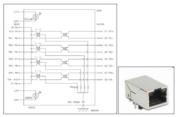
**Diagram 8: Ethernet Connector and Schematic**
